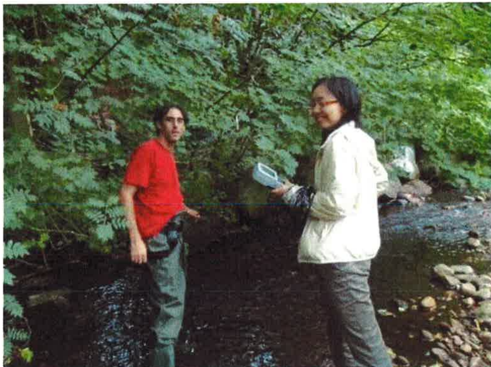
Photo 5 Using the YSI meter to measure water temperature, pH, dissolved oxygen and conductivity, August 2008 at MacKay Site 2. Britta Ng from District of North Vancouver joined us.
